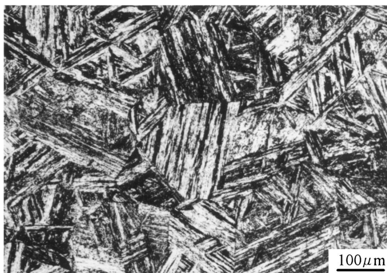
Figure 4 Microstructure of the specimen quenched at 313 K after solution treatment and then aged at 753 K for 14.4 ks.
